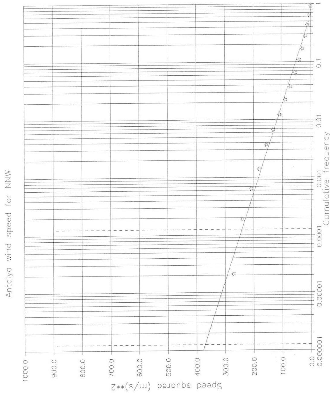
Fig.A-16. Cumulative frequency plot of Wind for NNW.
