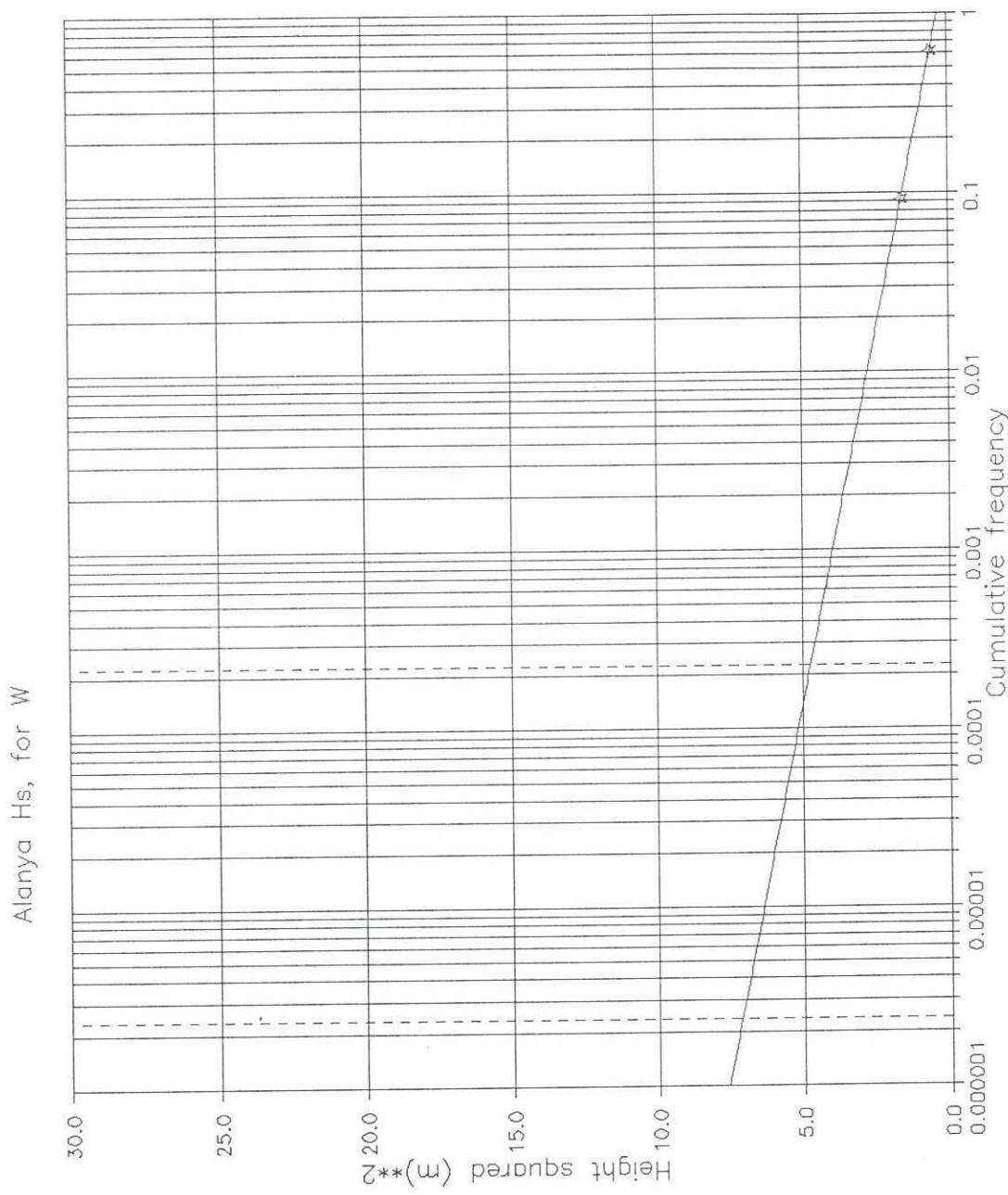
Fig.A-19. Cumulative frequency plot of H<sub>s</sub> for W.
