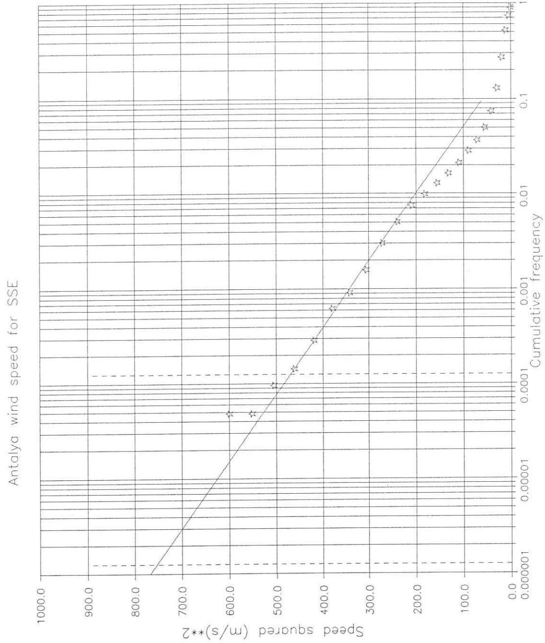
Fig.A-8. Cumulative frequency plot of Wind for SSE.
