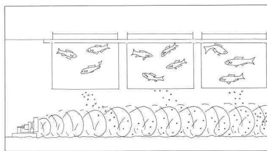
Fig. 2. Diagram of low-speed mixer installed on the bottom of a cage site to disperse wastes. (BEVERİDGE 1987)
