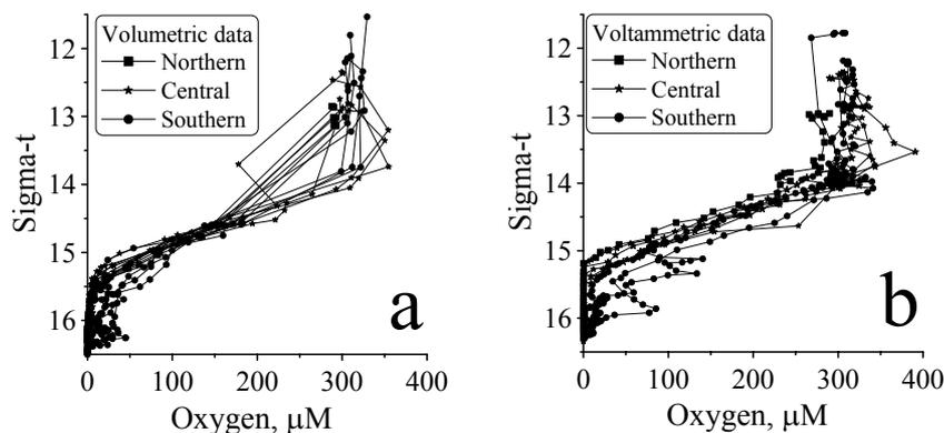
Fig. 2. Comparison of oxygen data determined by the volumetric (a) and voltammetric (b) methods.
