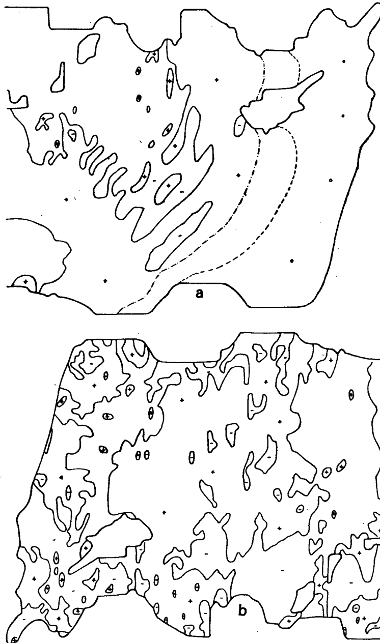
FIG. 3. The tsunami propagation pattern (a) at t = 4000 s and (b) at t = 60\,000 s.
