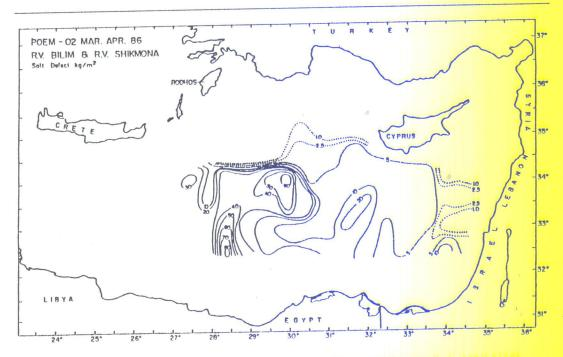
Fig. 23b. Negative salt anomaly in units of kg m<sup>-2</sup> calculated relative to a salinity upper limit of 39.0, MA86.
