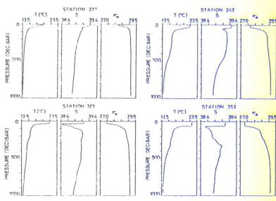
Fig.5. Selected profiles of temperature, salinity and density ( $\sigma_0$ ), ON85 cruise.
