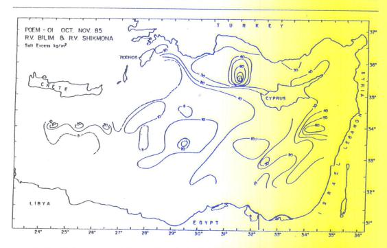
Fig. 22c. Positive salt anomaly in units of kg m<sup>-2</sup> calculated relative to a salinity lower limit of 38.9, ON85.
