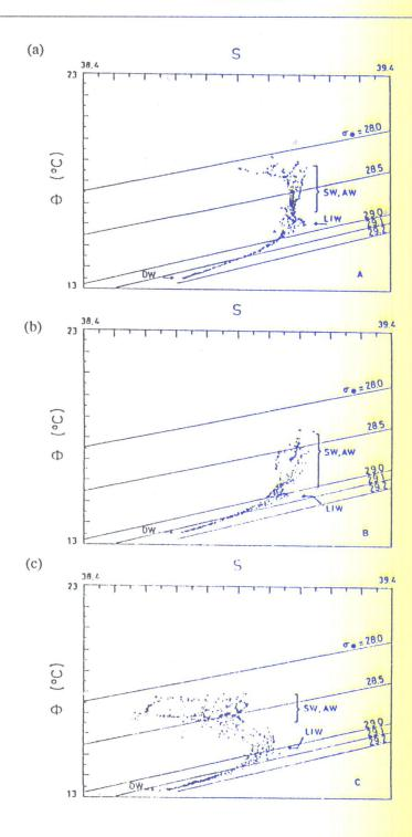
Fig.14. Potential temperature (Θ) and salinity (S) relationships for clusters of stations in areas (a) A, (b) B, and (c) C marked in Fig.2b, MA86.
