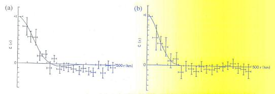
Fig.A1a,b. The experimental correlations showing the 90% confidence limits and the least squares fitted model for surface geopotential anomaly, (a) ON85, (b) MA86.
