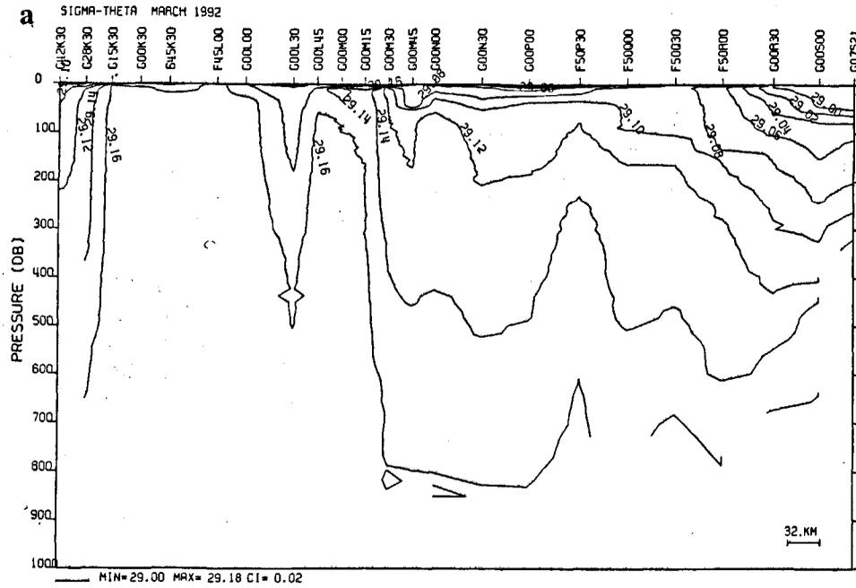
a) Density ( $\sigma_\theta$ ); b) salinity; and c) potential temperature ( $\theta$ ) distribution along transect of Figure 2 a during March 1992; and d) Density ( $\sigma_\theta$ ); e) salinity; and f) potential temperature ( $\theta$ ) distribution along transect of Figure 2 b in October 1991.
