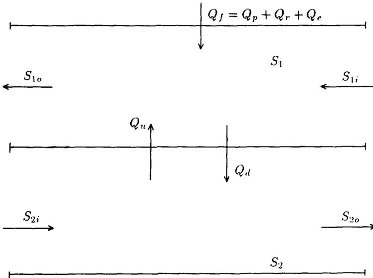
FIG.5. Compartment flows in a two-layer system.
