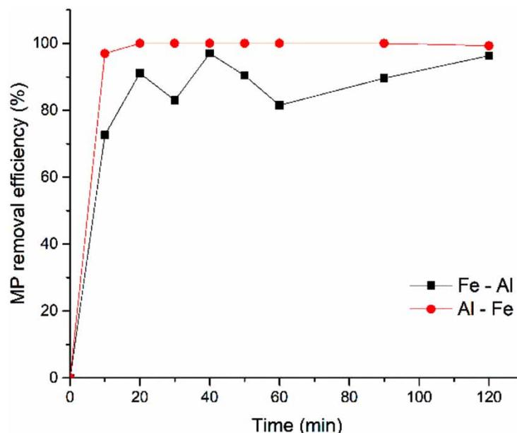
**Figure 4** | Microplastic (MP) removal efficiency via time with an initial concentration of 0.2 MPs/mL; pH 7; electrode distance 20 mm; and current density 15 A/m<sup>2</sup> in distilled water.
