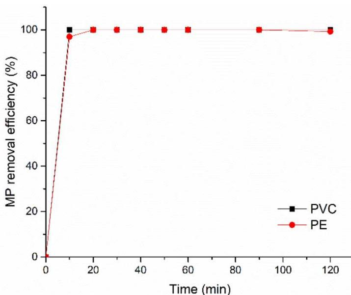
**Figure 7** | Microplastic removal efficiency for the two polymer types.
