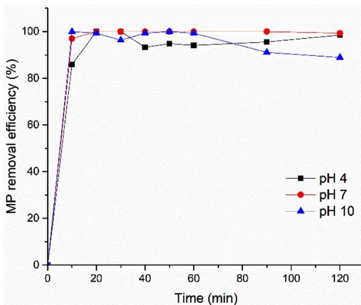
**Figure 5** | Microplastic removal efficiency via time with an initial concentration of 0.2 MPs/mL; electrode pair Al-Fe; electrode distance 20 mm; and current density  $15 \text{ A/m}^2$  in distilled water.
