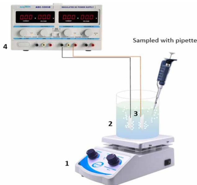
**Figure 1** | Schematic illustration of the EC/EF reactor (1. Magnetic stirrer, 2. EC/EF reactor, 3. Anode and cathode, 4. DC power supply).
