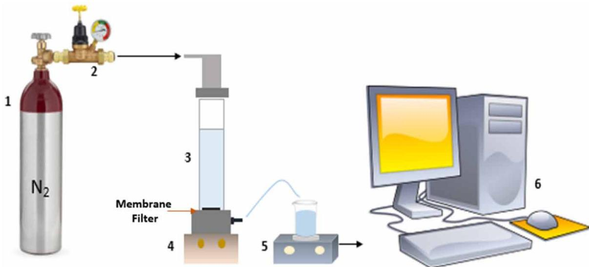
**Figure 2** | Schematic illustration of dead-end filtration unit (1. Nitrogen gas tank, 2. Pressure regulator, 3. Dead-end reactor, 4. Magnetic stirrer, 5. Precision balance, 6. Computer).
