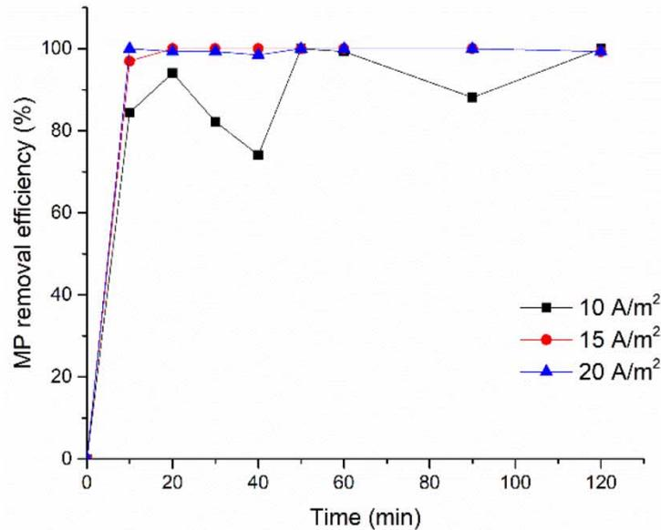
**Figure 6** | Microplastic removal efficiency via time with initial concentration of 0.2 MPs/mL; electrode pair Al-Fe; electrode distance 20 mm; current density 15 A/m<sup>2</sup>; and pH 7 in distilled water.
