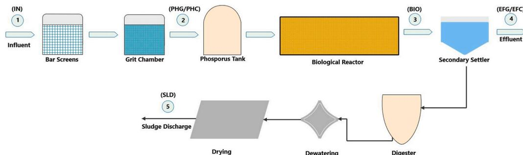
Fig. 1. Flow diagram of WWTP and sampling points (Modified from Akarsu et al., 2020).
