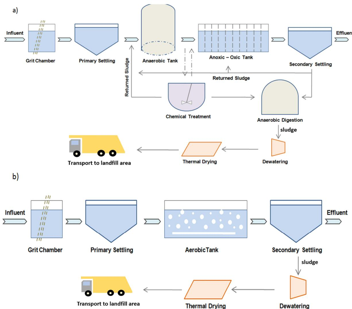
Fig. 2. Schematic diagram of Karaduvar WWTP (a, tertiary treatment), and Silifke & Tarsus WWTPs (b, secondary treatment).
