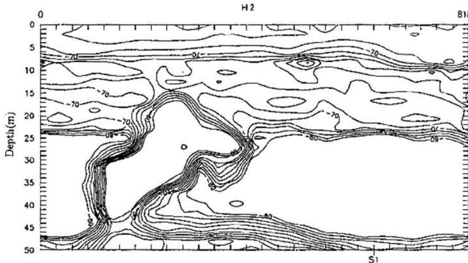
**Figure 3.** Absolute backscatter measured by the on-board ADCP of the R/V BİLİM near the Ahırkapı diffuser on 18 May 1992.
