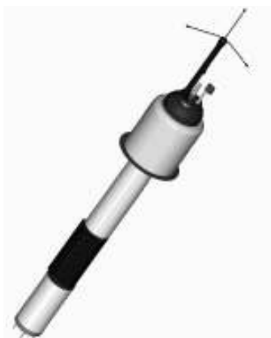
Figure 4 The Pagode coastal profiler (under development, preliminary profiles with a prototype).
