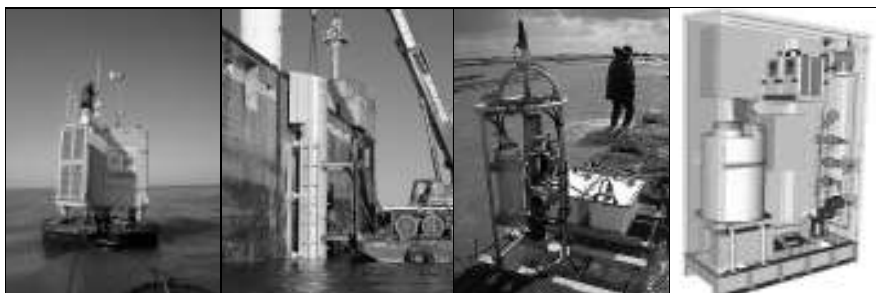
Figure 3 Marel water quality automatic monitoring concept (buoy, pier, aquaculture, Ferrybox).
