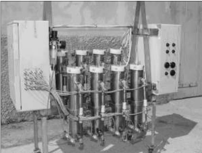
Figure 1 The multiple launcher with the electro-valves box (left) and the electronics box (right).
