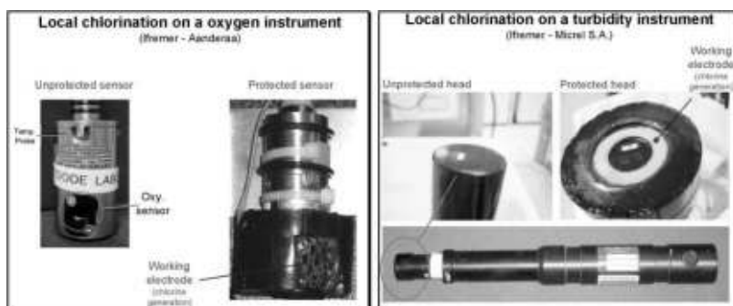
Figure 2 Local chlorination on oxygen optode (left) and on turbidity sensor (right).
