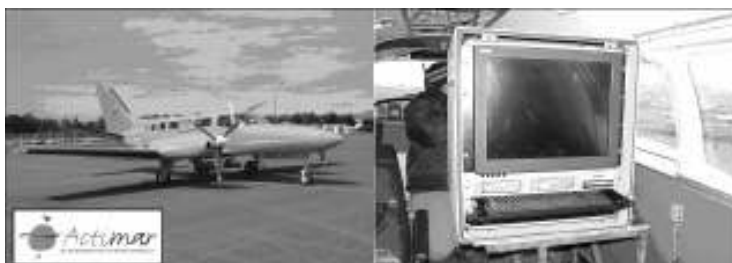
Figure 5 Aircraft equipped for laser surveys and inside racks.
