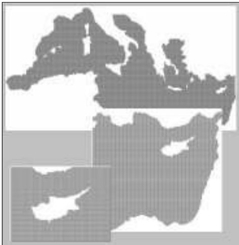
Figure 3 The Cyprus Wave Model forecasts wave height and direction for the entire Mediterranean. Nested within that model is the wave forecast for the Levantine basin (inset 1). Nested within the WAM is a high-resolution SWAN model (inset 2).
