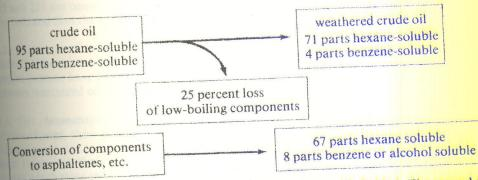
which is equivalent to 88 % hexane-soluble, in approximate agreement with Table 1. The second reaction, which in fact occurs simultaneously with the first, is a representation of the small chemical changes that sehave shown to be caused by weathering.
