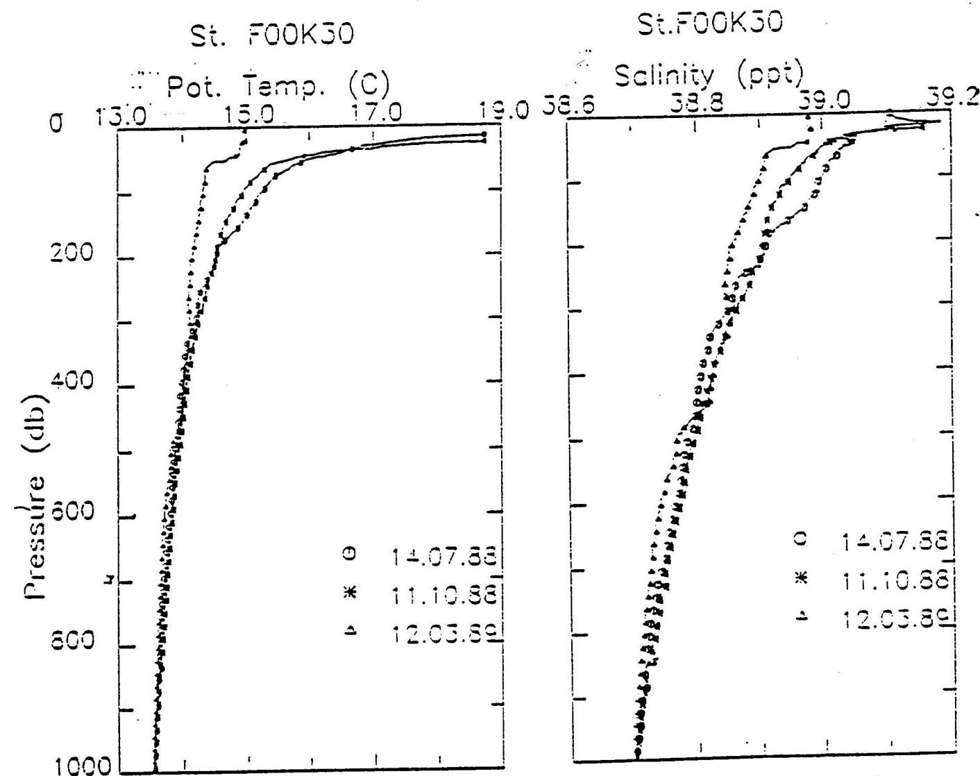
Fig. 5 The observed vertical profiles of the temperature and salinity at station F00K30 situated within the quasi-permanent Rhodes cyclonic region at different times of a year.
