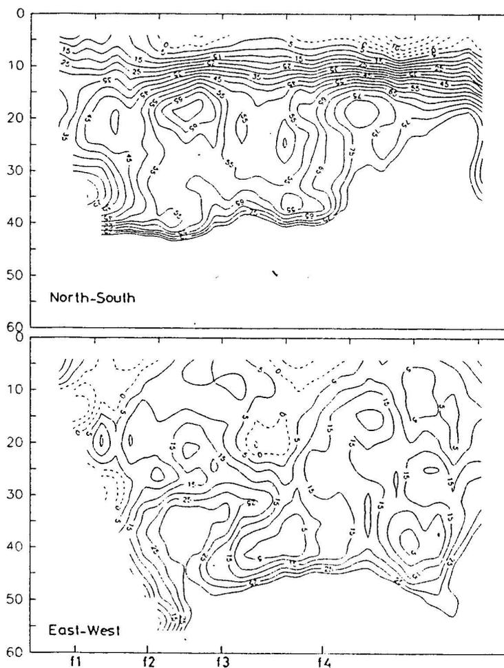
Fig. 5. The ADCP derived velocities along section 1 across the Ahırkapı diffuser pipeline, 4 March 1993. Upper panel shows north-south component of the velocity and positive indicate north (solid line). Lower panel shows east-west component of the velocity and positive indicate east (solid line).
