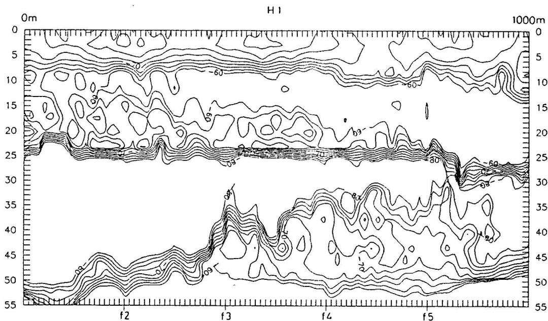
Fig. 3.b. Absolute acoustic backscatter(db) recorded along section 1 across Ahirkapi diffuser pipeline, 18 May 1992.
