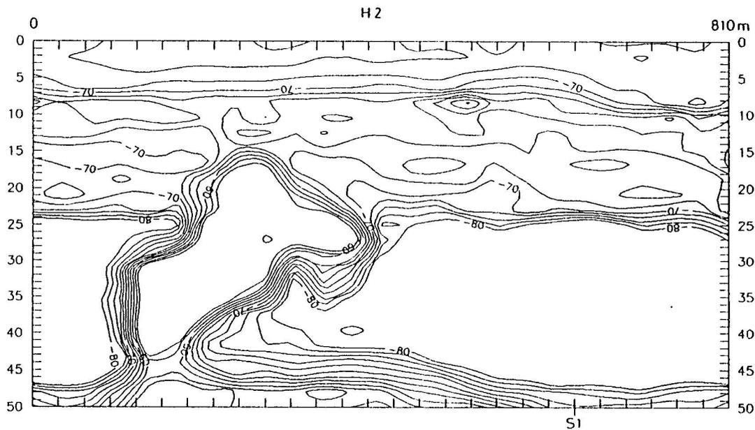
Fig. 4.b Absolute acoustic backscatter(db) recorded along section 2 across Ahirkapi diffuser pipeline, 18 May 1992.
