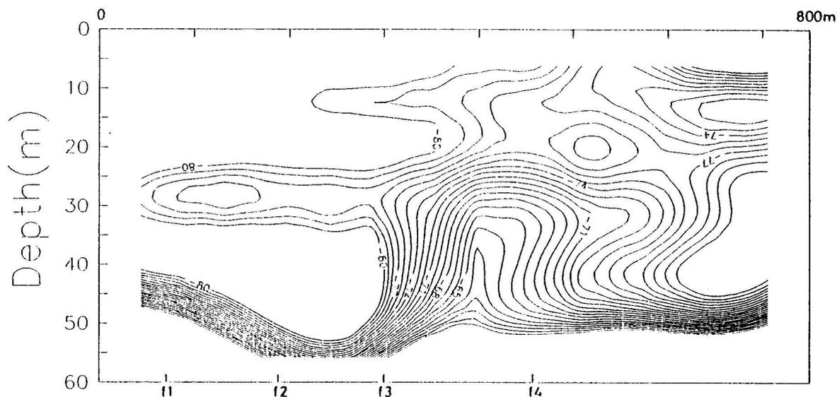
Fig. 7.b Absolute acoustic backscatter(db) recorded along section 1 across Ahirkapi diffuser pipeline, 4 March 1993.
